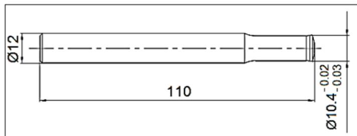
*Figure 2. Technical drawing of a coated piercing punch*
