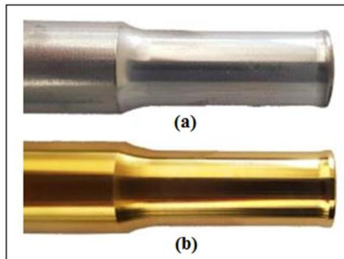
*Figure 1. (a) uncoated and (b) coated AISI M2 piercing punches*
