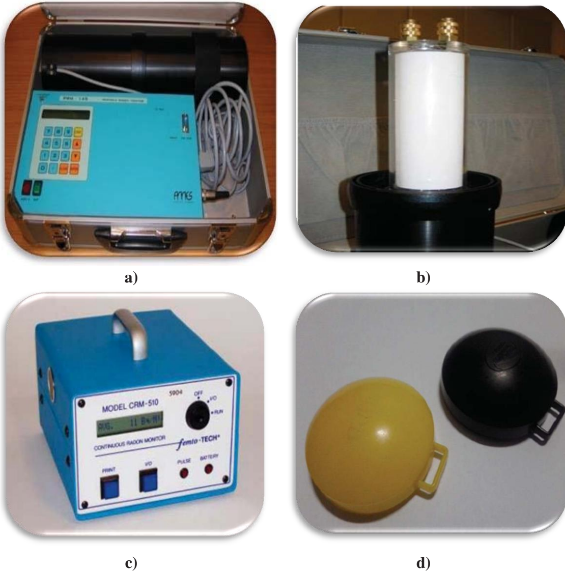
Fig.1. a) PRM 145 device with b) scintillation cells, c) CRM-510 device for continuous monitoring and d) track detectors used for radon measurements.
