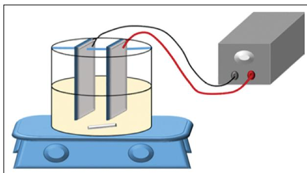
**Figure 1.** Schematic representation of EC in the laboratory.
