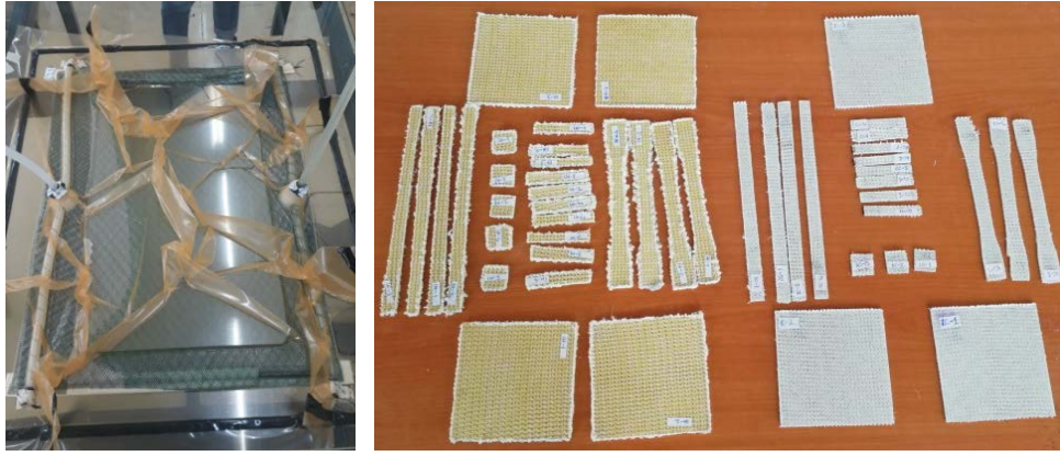
Figure 2. The composite production via vacuum infusion (left), the composite panel specimens (right)
