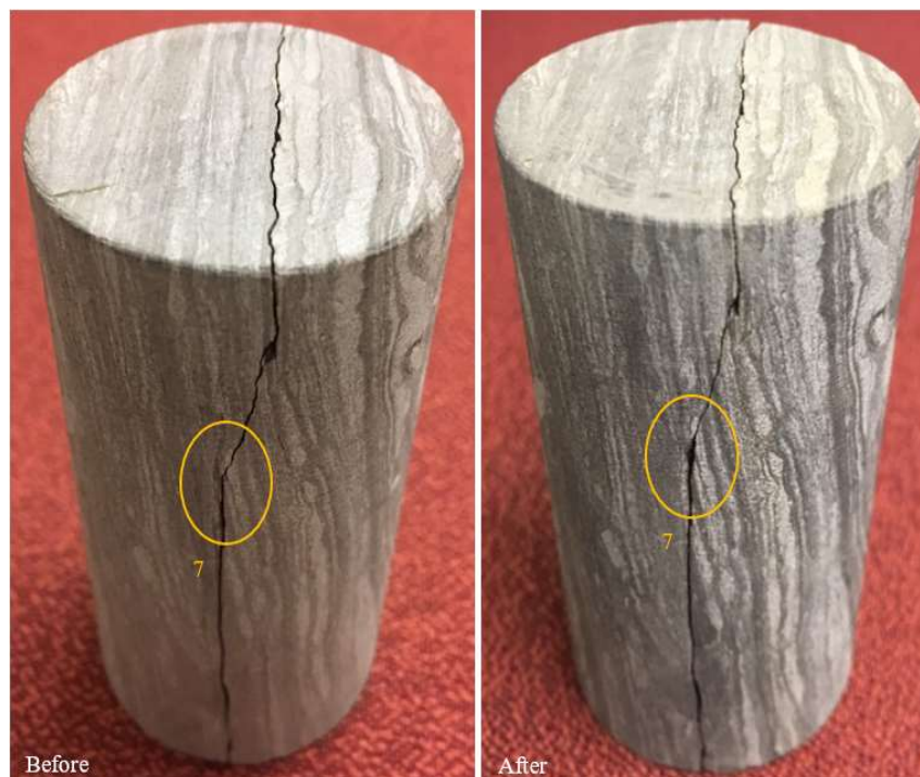
Fig. 9. Comparison of the cylindrical side surface of Mancos Shale sample
