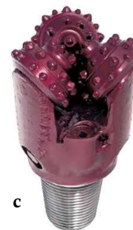
Fig. 32. Rates of penetration and costs of meter for IADC 517 tricone bits used in the formations in Southeastern Anatolia and Thrace Basins; a) relationship between average net penetration rates and formations, b) relationship between net penetration rates and costs of meter, c) view of an IADC 517 tricone bit
