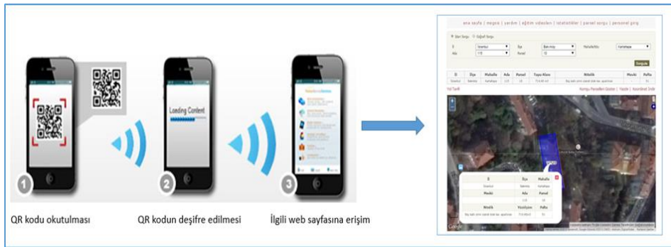
Figure 12. Scanning title deed printed QR code and accessing related URI address.
