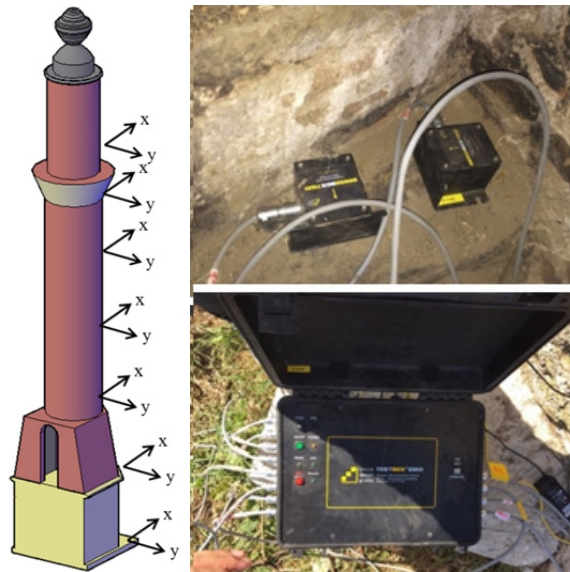
Figure 7. Locations and directions of the accelerometers on the minaret and data acquisition system.
