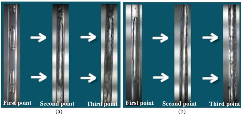
**Figure 5.** Two-phase flow regimes under a and b conditions
