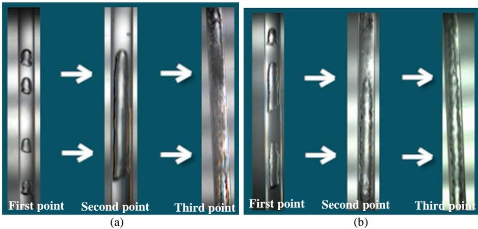
**Figure 4.** Two-phase flow regimes under a and b conditions
