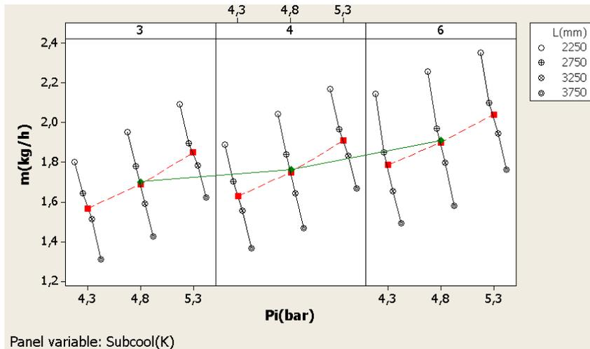
**Figure 6.** The variation of the mass flow rate under different capillary tube inlet pressures, capillary tube lengths and subcooling degrees
