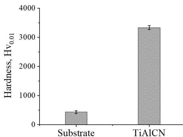
**Figure 6.** The hardness values of substrate ve TiAlCN coated samples
