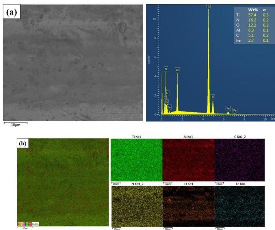
**Figure 9.** Taken from the wear area of the TiAlCN coated sample; a) SEM image and EDX analysis and b) EDX map results
