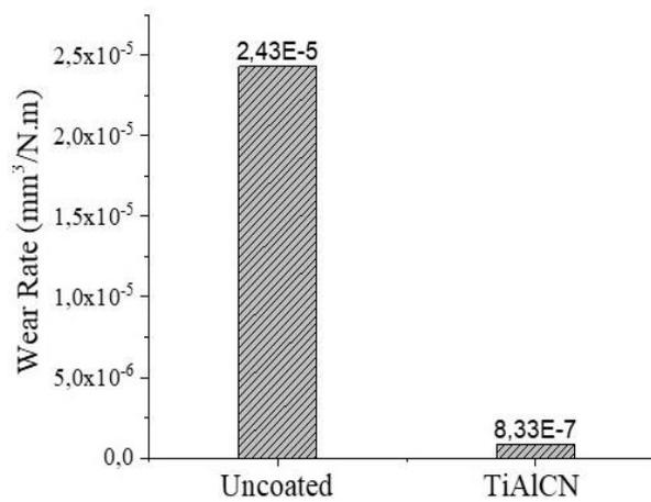
**Figure 11.** Wear rates of uncoated and TiAlCN coated samples
