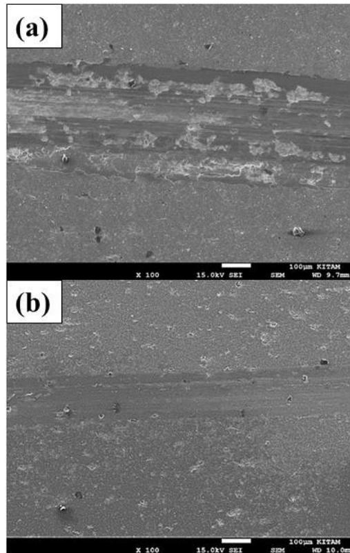
**Figure 10.** SEM images of wear scars a) Uncoated and b) TiAlCN
