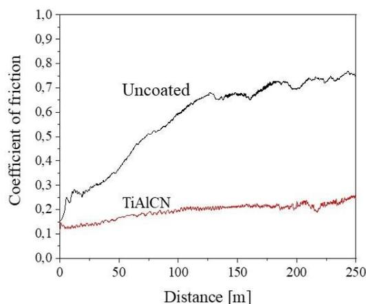
**Figure 7.** Coefficients of friction of uncoated and coated piston rings
