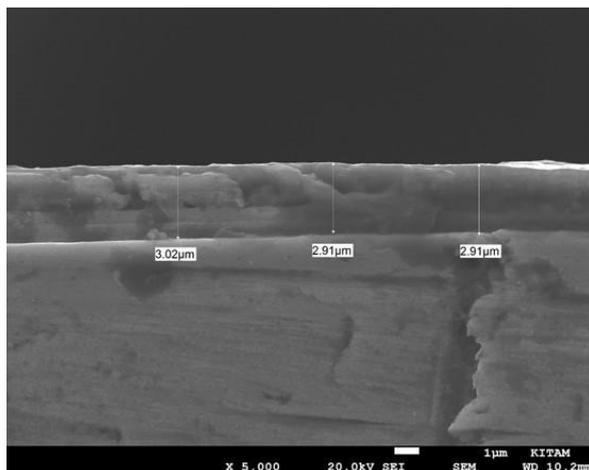
**Figure 4.** SEM image of the coating TiAlCN
