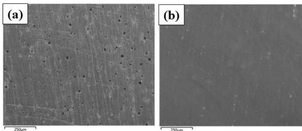
**Figure 3.** SEM surface morphologies of samples a) uncoated, b) TiAlCN
