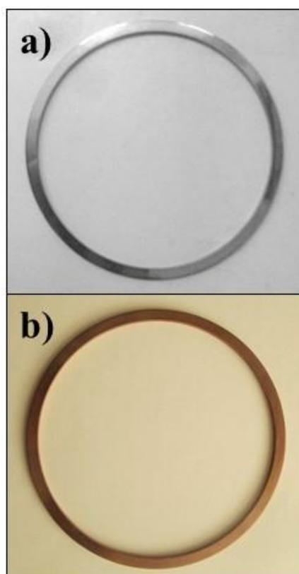
**Figure 1.** Piston rings a) uncoated and b) TiAlCN coated
