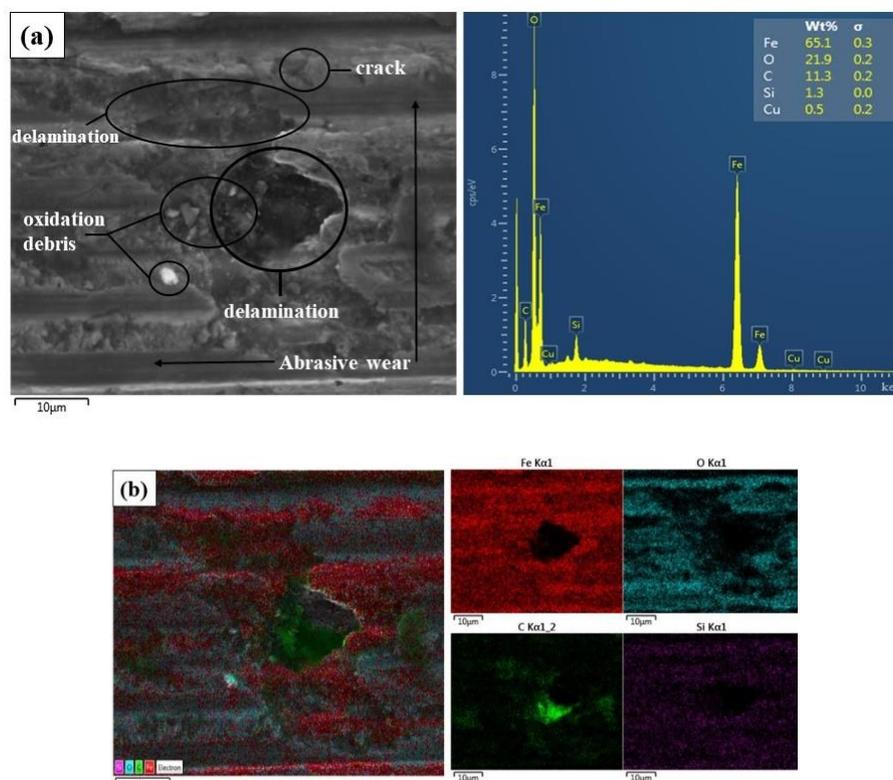
**Figure 8.** Taken from the wear area of the uncoated sample; a) SEM image and EDX analysis and b) EDX map results
