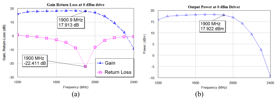
Figure 3 a, b. Simulation Result of PA without MC, Output power at 0 dBm without MC
