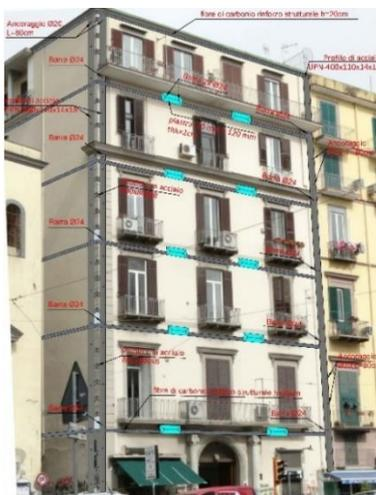
**Figure 40.** Rendering of some of the structural reinforcing on the external wall of the building
