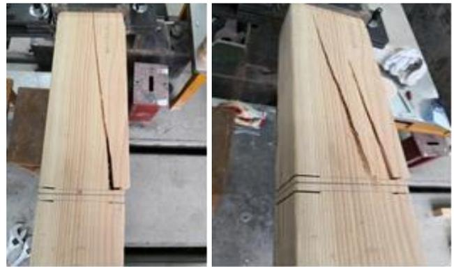
Figure 9. Midspan failure of S2 group
