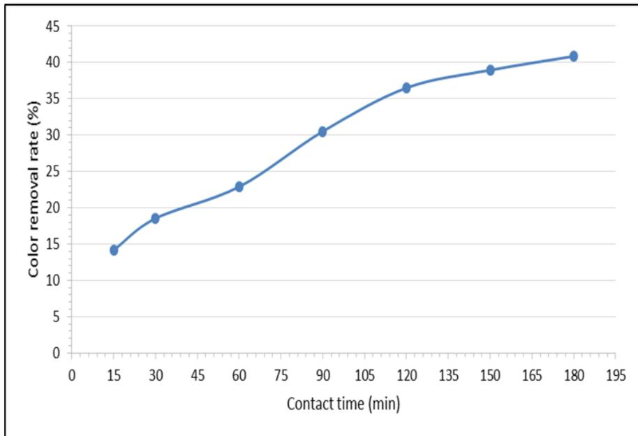
**Figure 3.** Effect of contact time on color removal efficiency for WMH
