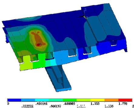
Figure 4. Distribution of deformation vector sum for rib web slope of 87.92°. Max. value is 1.898 mm.
