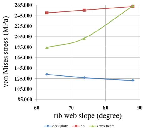
**Figure 11.** Variation of max.von Mises stress depending on slope of rib web.
