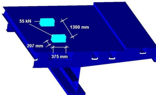
Figure 3. Wheel loads on quarter of bridge' s FE- model.
