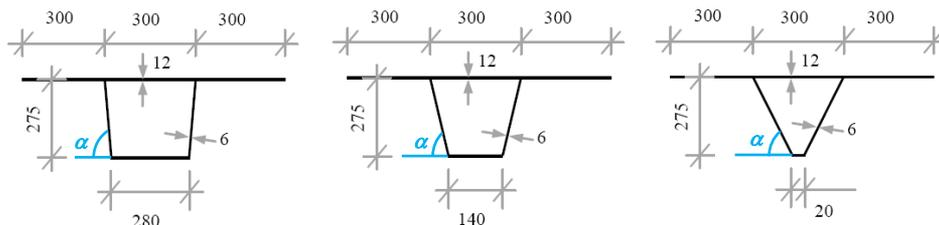
**Figure 1.** Dimensions (in mm) of different rib shapes used in this study. The slopes of the rib shapes from left to right are  $87.92^\circ$ ,  $73.78^\circ$  and  $63.02^\circ$  respectively.
