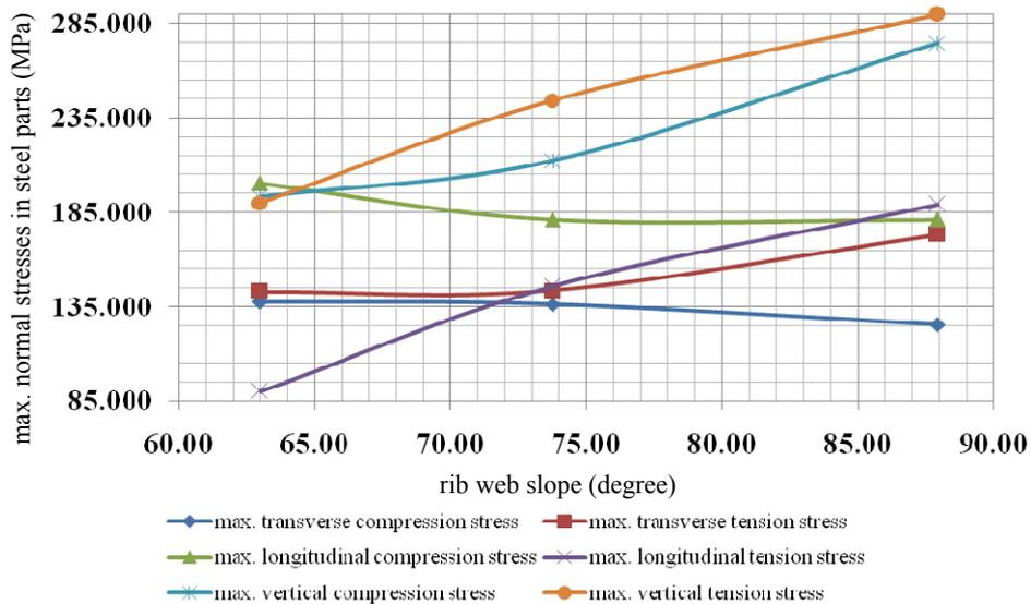
**Figure 12.** Variation of max. stresses in steel parts depending on slope of rib web.
