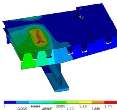
Figure 5. Distribution of deformation vector sum for rib web slope of 73.78°. Max. value is 1.729 mm.
