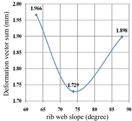
Figure 7. Variation of deformation vector sum depending on rib web slope.
