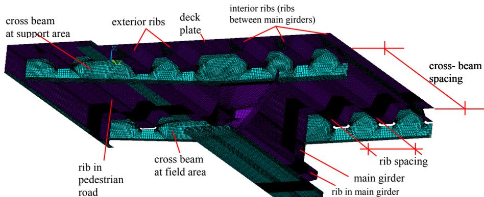
**Figure 2.** FE- model of orthotropic steel bridge.
