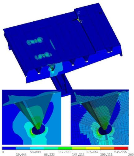
**Figure 10.** Distribution of von Mises stress with averaged nodal values (top and bottom left) and non- averaged elemet results (bottom right) for rib web slope of 63.02°. Max. values developed in deck plate, ribs and cross beams are 132.997 MPa, 250.202 MPa and 184.319 MPa respectively.
