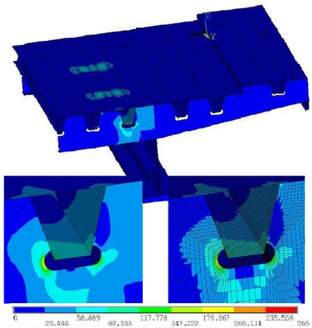
**Figure 9.** Distribution of von Mises stress with averaged nodal values (top and bottom left) and non- averaged elemet results (bottom right) for rib web slopeof 73.78°. Max. values developed in deck plate, ribs and cross beams are 126.652 MPa, 255.259 MPa and 201.549 MPa respectively.
