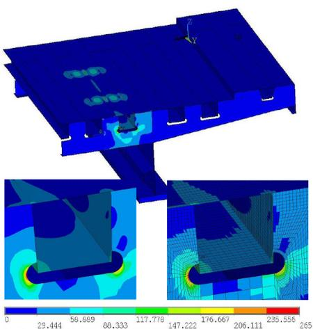
**Figure 8.** Distribution of von Mises stress with averaged nodal values (top and bottom left) and non- averaged elemet results (bottom right) for rib web slope of 87.92°. Max. values developed in deck plate, ribs and cross beams are 121.538 MPa, 262.34 MPa and 263.612 MPa respectively.
