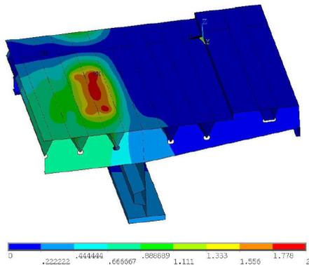
Figure 6. Distribution of deformation vector sum for rib web slope of 63.02°. Max. value is 1.966 mm.
