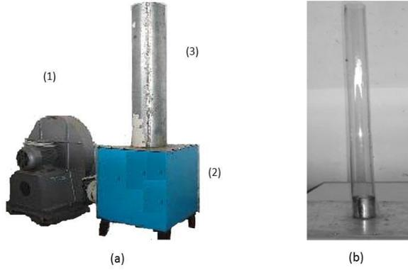
Figure 1. Experimental set up (a): 1, centrifugal fan; 2, air distribution room; 3, cylindrical container, (b): The transparent cylindrical pipe used for the test of terminal velocity.
