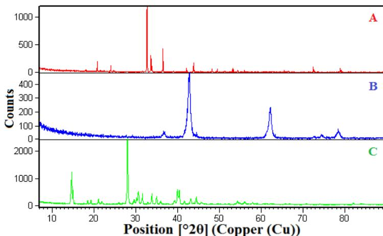
Figure 1. Raw materials XRD patterns; A.  $\text{MgCl}_2 \cdot 6\text{H}_2\text{O}$ , B.  $\text{MgO}$ , C.  $\text{H}_3\text{BO}_3$
