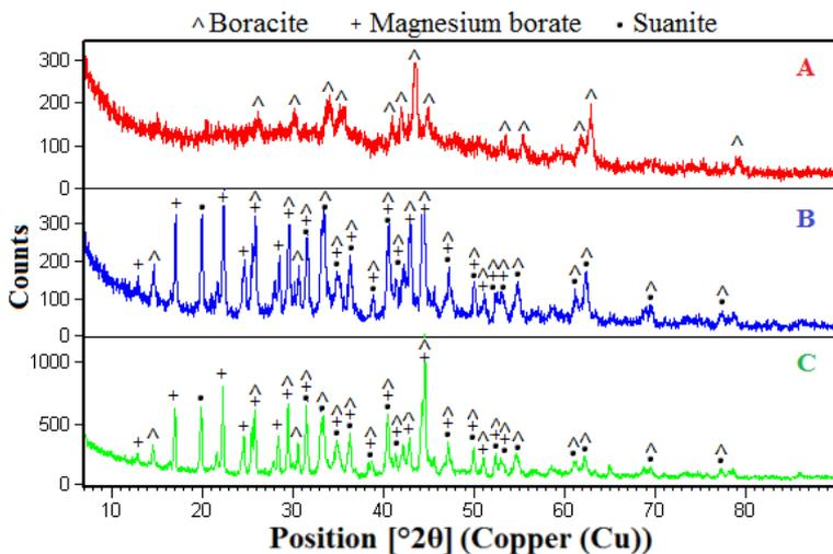
Şekil 4. 1-6-13 ratio raw materials XRD patterns obtained at; A.  $500^\circ\text{C}$ , B.  $600^\circ\text{C}$ , C.  $700^\circ\text{C}$
