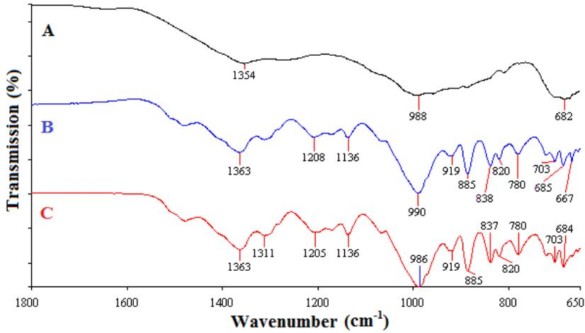
Şekil 5. 1-4-13 ratio raw materials FT-IR spectra obtained at; A. 500°C, B. 600°C, C. 700°C
