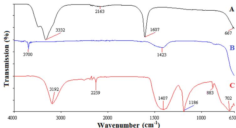
Figure 2. Raw materials FT-IR spectra; A.  $\text{MgCl}_2 \cdot 6\text{H}_2\text{O}$ , B.  $\text{MgO}$ , C.  $\text{H}_3\text{BO}_3$
