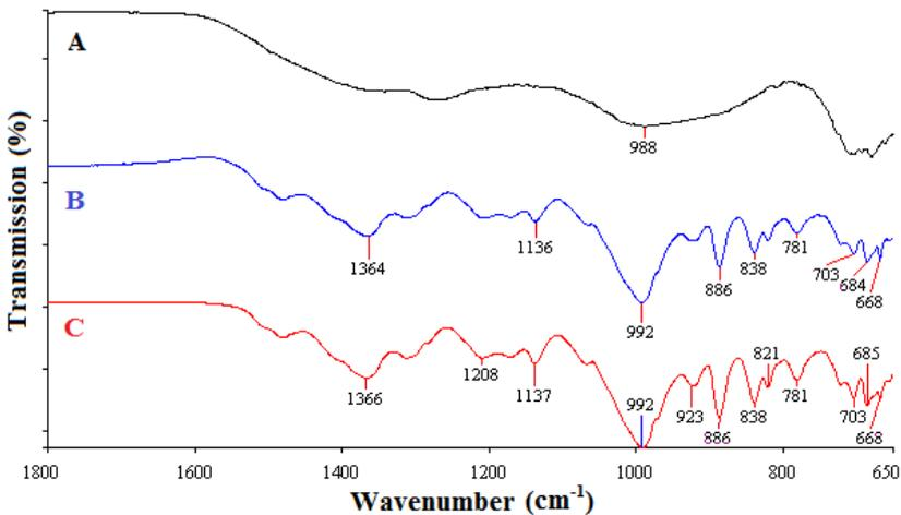
Şekil 6. 1-6-13 ratio raw materials FT-IR spectra obtained at; A. 500°C, B. 600°C, C. 700°C
