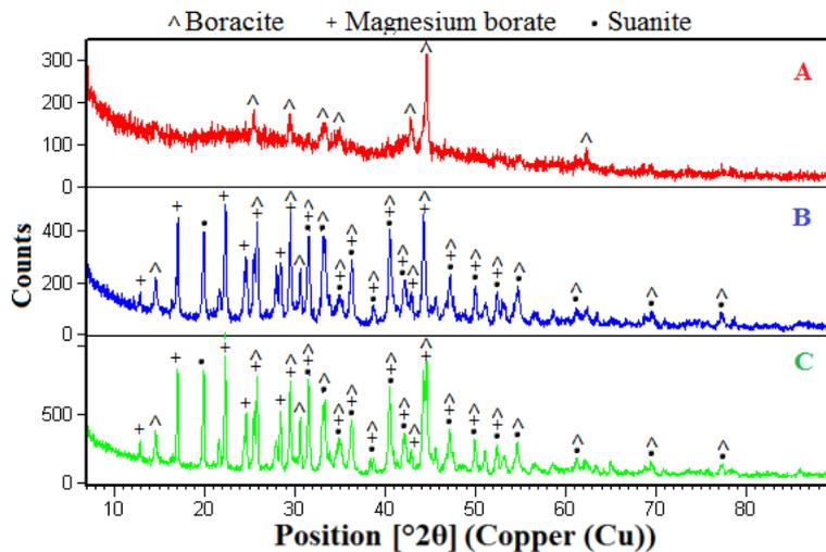
Figure 3. 1-4-13 ratio raw materials XRD patterns obtained at; A.  $500^\circ\text{C}$ , B.  $600^\circ\text{C}$ , C.  $700^\circ\text{C}$
