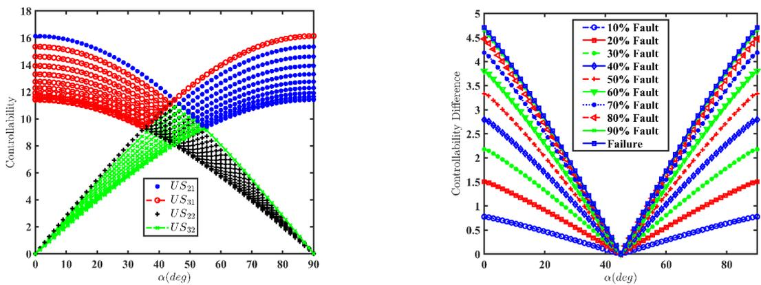
Figure 8. Different magnitudes of fault on number two motor
