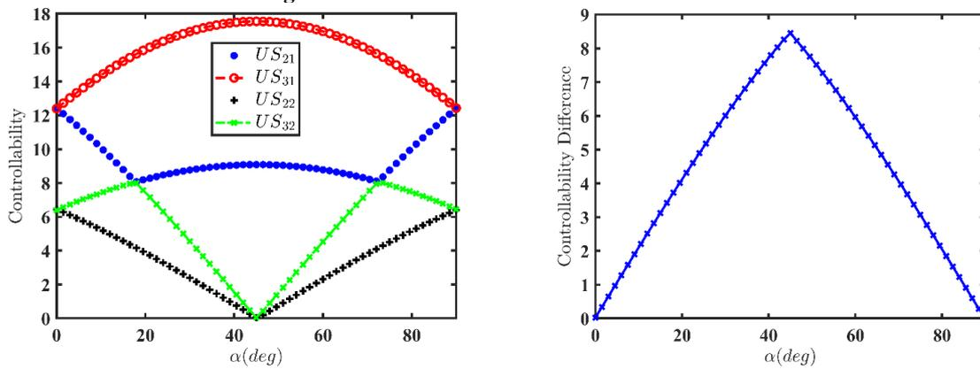
Figure 17. Failure of number one, three, and six motors
