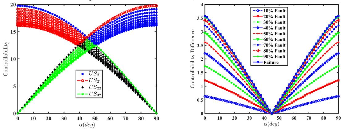
Figure 18. Different magnitudes of fault on number one motor
