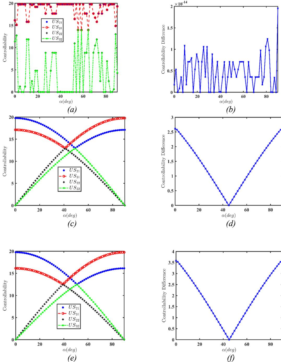
**Figure 9.** Variation of controllability parameters and the controllability difference ( $J$ ) for quadrotor
