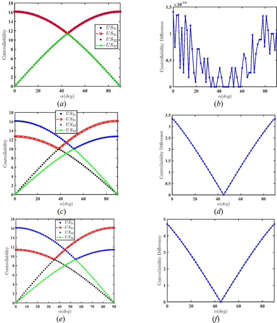
**Figure 5.** Variation of controllability parameters and the controllability difference ( $J$ ) for quadrotor (a, b) No rotor failure, (c, d) 50% fault on rotor number 1, (e, f) failure on rotor number one
