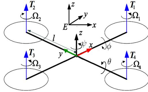
Figure 2. Schematic representation of quadrotor
