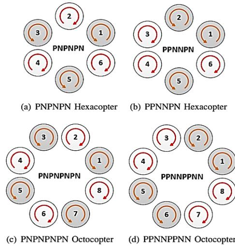
**Figure 4.** Hexarotor and octarotor with traditional arrangement of rotors and non-standard rotors
