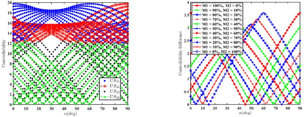
Figure 21. Different magnitudes of fault on number one and two motors
