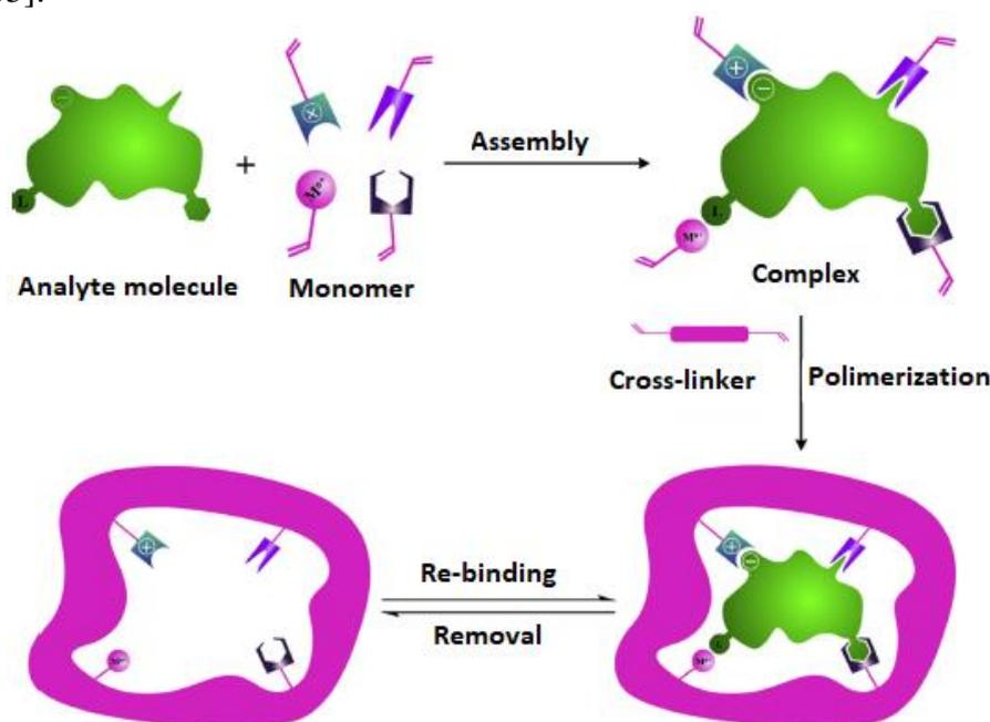
**Figure 4.** The preparation of molecular imprinted polymers [36]
