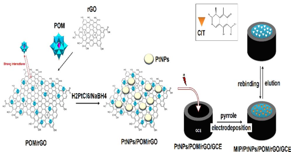
**Figure 5.** The development of CIT- imprinted sensor [37]
