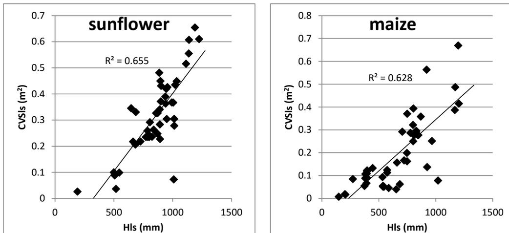
**Figure 7.** Correlations between plants height (Hls) and Canopy Vertical Surface (CVSls) for the data obtained with the laser scanner sensor for sunflower and maize.
