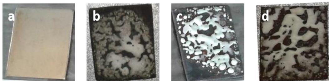
**Figure 3.** The photographs of non-coated Cr steel sheet (a) and Cr steel coated with dehydrated glass powder at 950°C temperature for 1 hour (b), 2 hours (c) and 3 hours (d)
