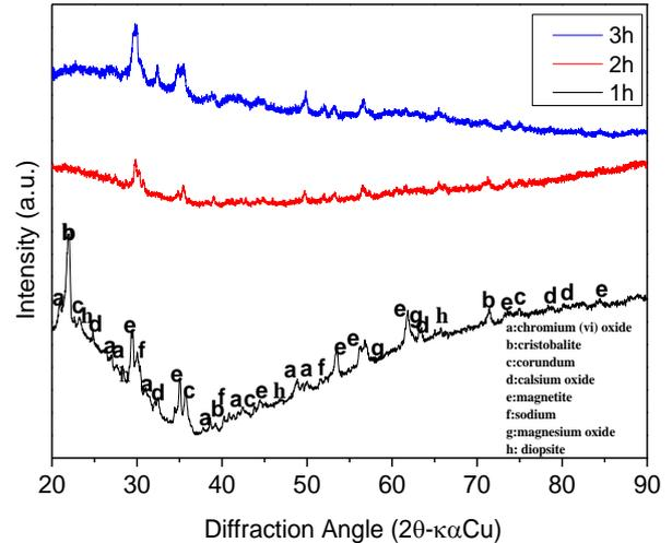
**Figure 7.** The XRD Patterns of Cr steel sheet coated with dehydrated glass powder at 950 °C temperature for 1 ,2, and 3 hours.
