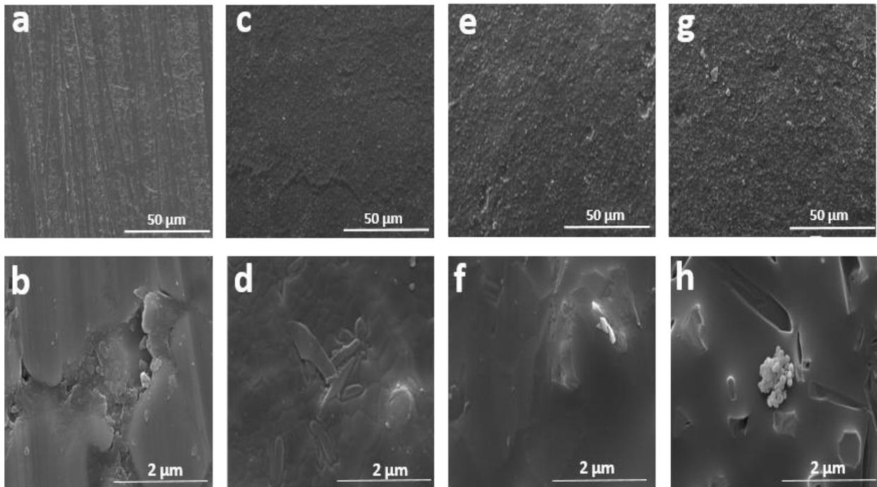
**Figure 5:** The SEM images of non-coated Cr steel sheet (a, b) and Cr steel sheet coated with dehydrated glass powder at 950 °C temperature for 1 hour (c, d), 2 hours (e, f) and 3 hours (g, h)
