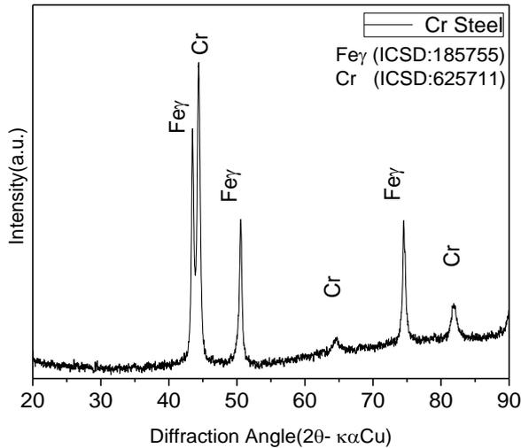
**Figure 6.** The XRD Pattern of non-coated Cr steel sheet.
