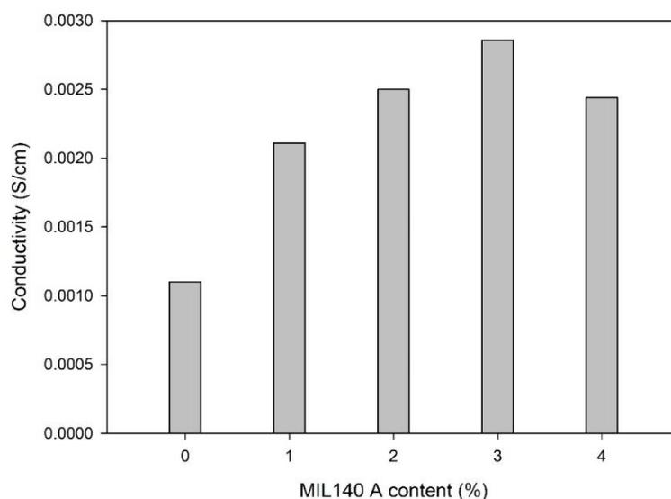
Fig. 5. Proton conductivity results of the membranes
