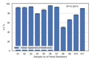
Figure 2. Alcohol amounts obtained as a result of HS/GC-MS Analysis of commercial hand sanitizers (ISA and ethanol, v/v%)
