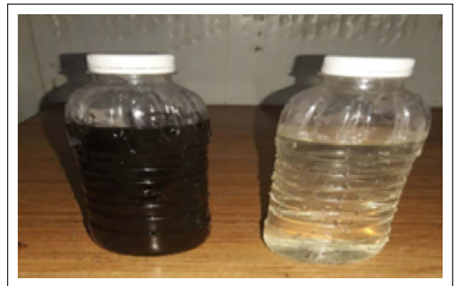
Figure 10. Raw leachate (on the left) and permeate (on the right).
