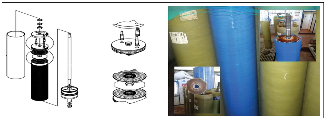
Figure 1. RO treatment plant membrane design and disc membranes.
