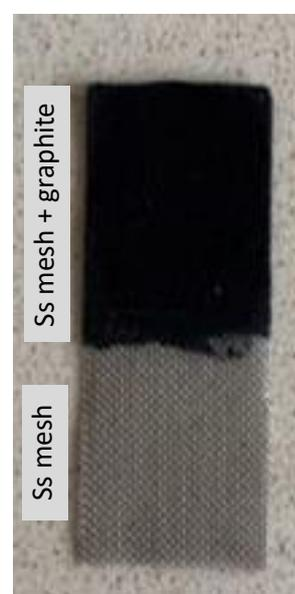
**Figure 3.** Stainless steel mesh + graphite electrode.
