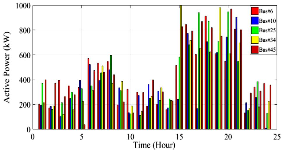
**Figure 6.** Production capacity of distributed generation units in twenty-four hours
