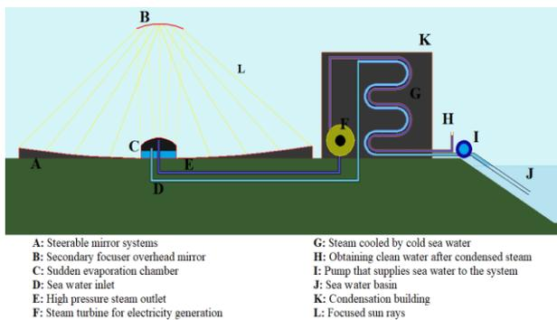
Fig. 4. Operating diagram of the MEW Plant
