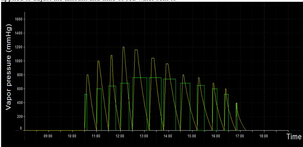
Fig. 9. Vapour pressure in sudden evaporation unit.
