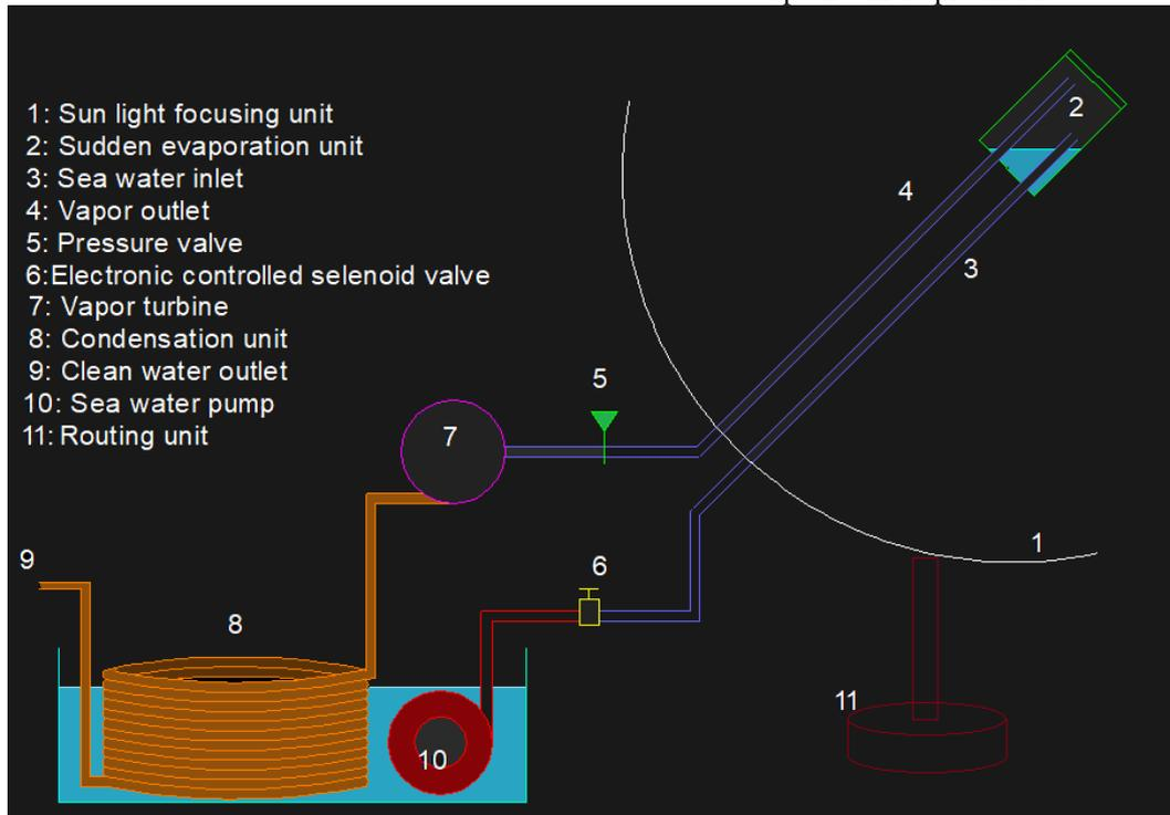
Fig. 5. Diagram of prototype system.
