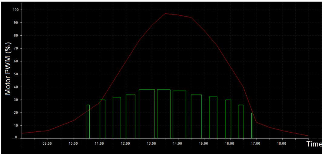
Fig.8. Sea water pump cycle
