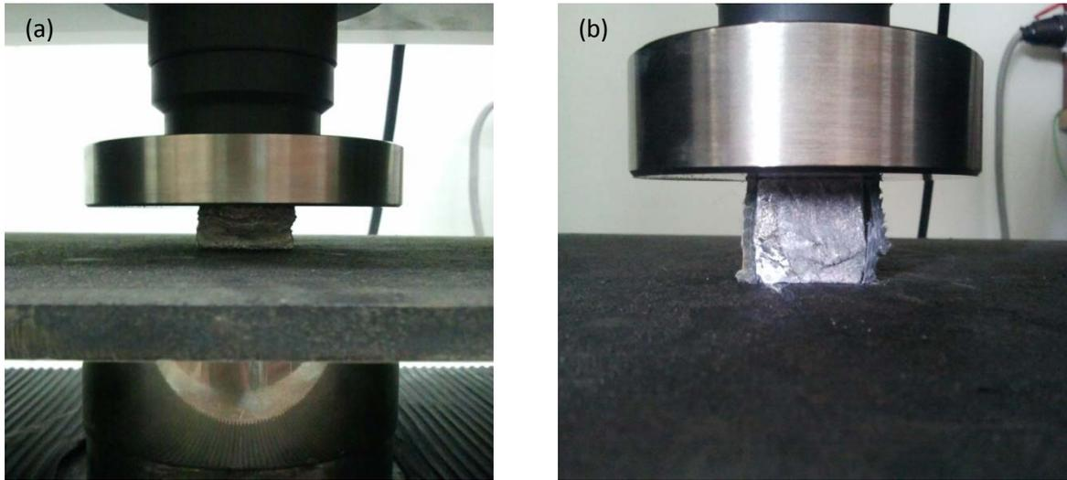
**Fig. 5.** Collapsed sandwich specimens during (a) flatwise compression with crushing and shear of the core (b) edgewise compression with crushing and shear of the core and debonding and buckling of facesheet.
