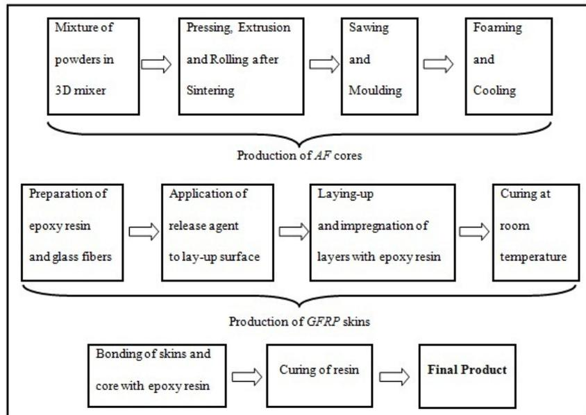
Figure 2. Illustration of production process of *GFR-AF* panels
