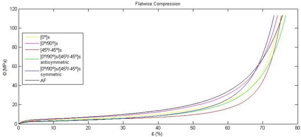
**Figure 3.** Stress-strain curves measured under static flatwise compression
