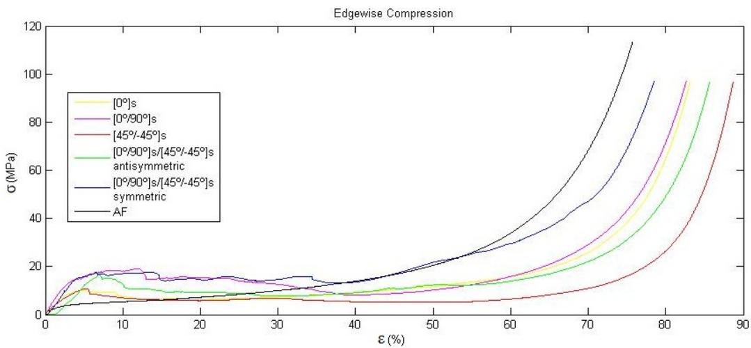
**Figure 4.** Stress-strain curves measured under static edgewise compression
