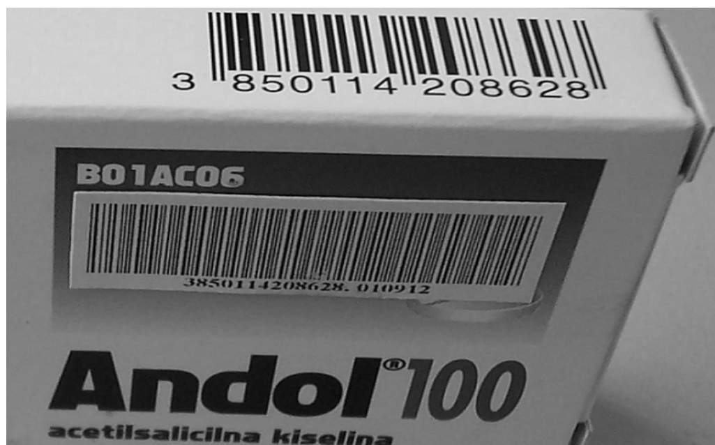
Picture 2. Sample of drug with extended barcode (front side) and EAN13 (top side)
