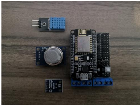
Figure 8. Sensor devices and NodeMcu with its motor shield
