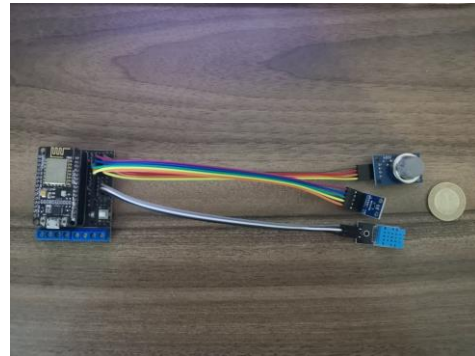
Figure 8. Sensor devices and NodeMcu with its motor shield
