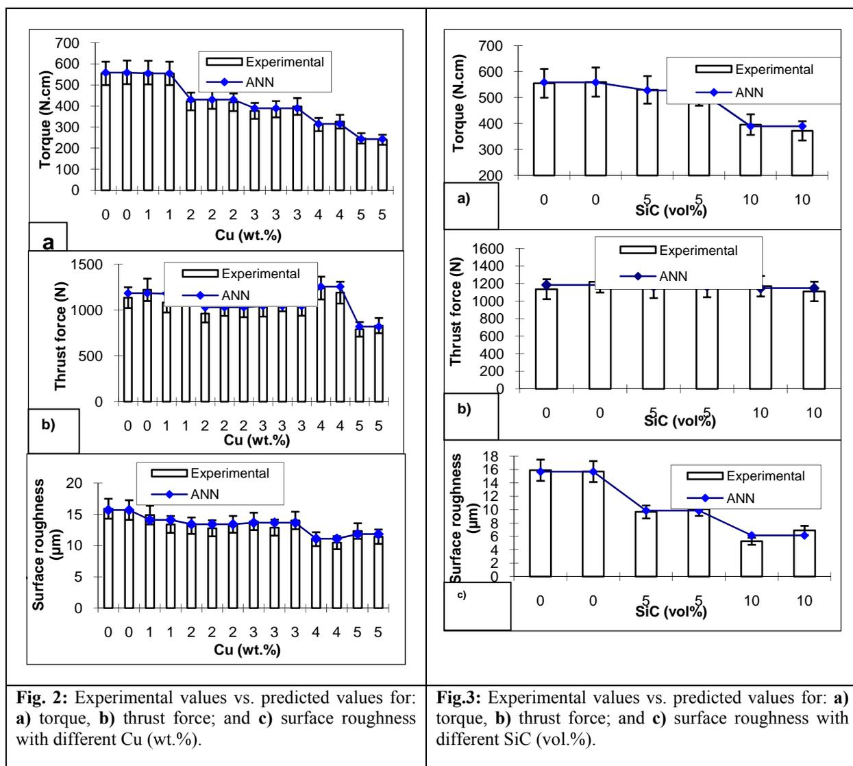
4.2 Effect of copper and silicon carbide addition on the drilling of aluminum
