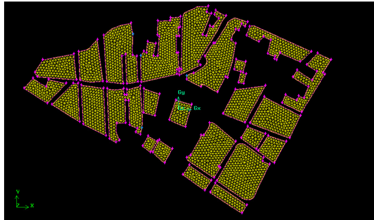
Fig.5 Triangular Paved Mesh on Flow-volume Bottom Face of the Urban Configuration
