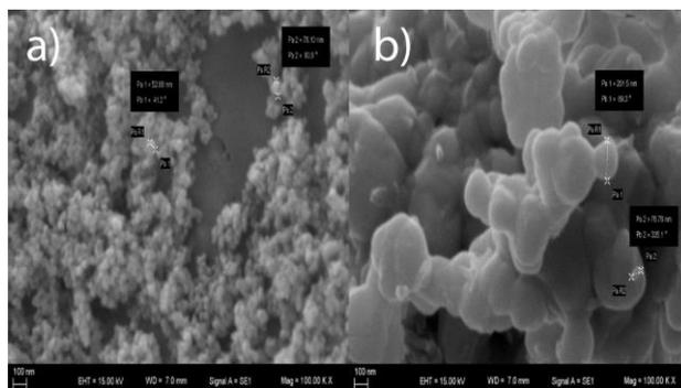
Figure 3. Scanning electron microscopy of (a) TiO<sub>2</sub> and (b) Ag NPs (100,00K X)
