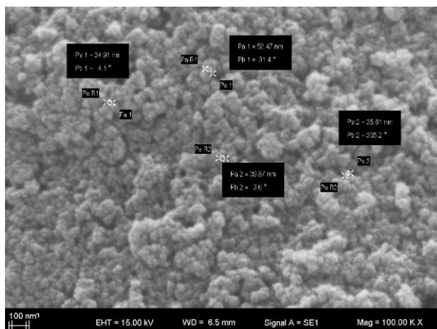
Figure 4. Scanning electron microscopy observation of TiO<sub>2</sub>@Ag NPs (100,00K X)
