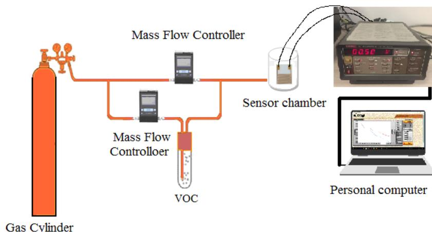
**Figure 2.** Schematic of the VOC vapor sensing configuration
