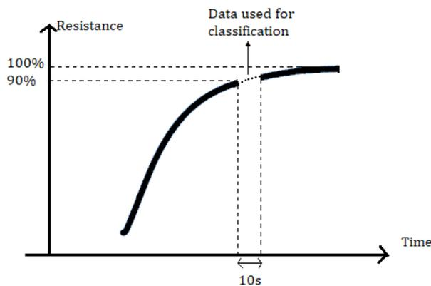
**Figure 4.** The feature extracted from each response curve
