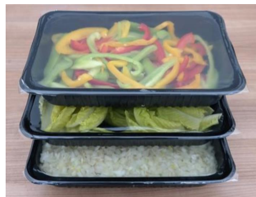
Figure 3. Heat sealable coated BOPET film food packaging application
