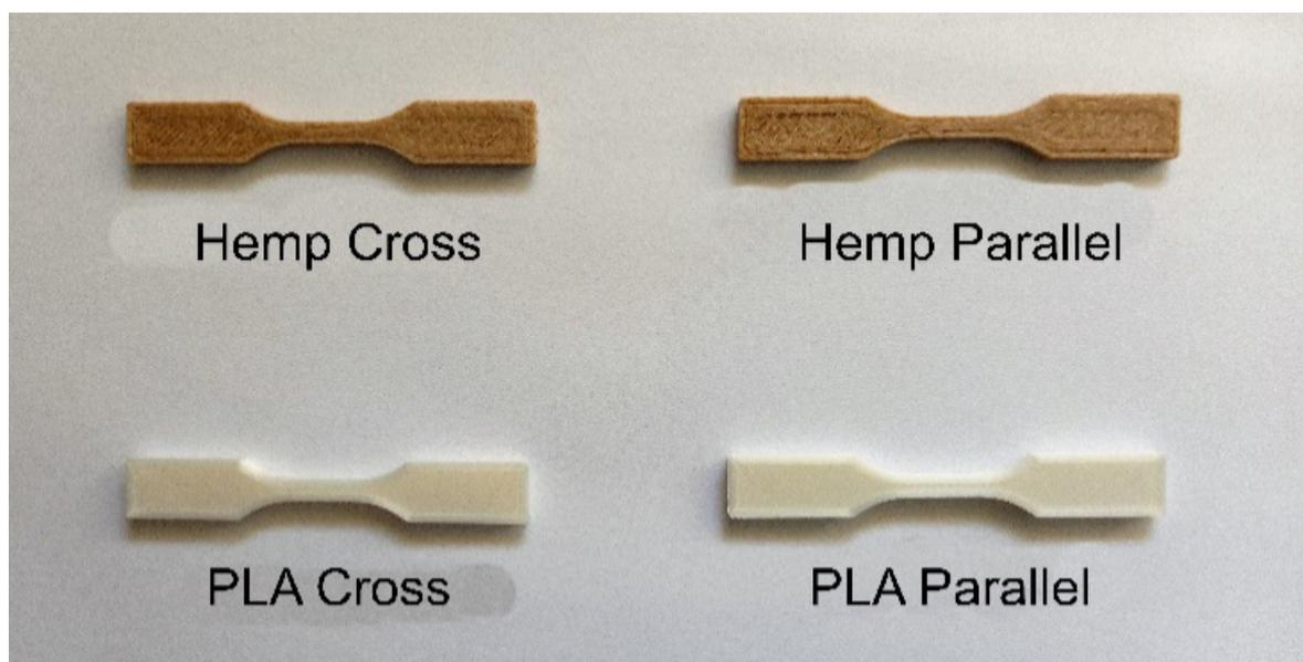
**Figure 3.** Tensile test specimens.
