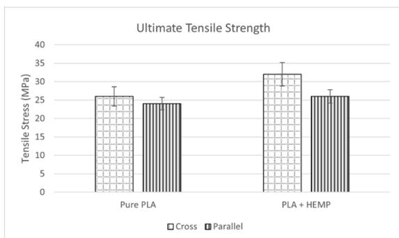
Figure 8. Tensile test results.
