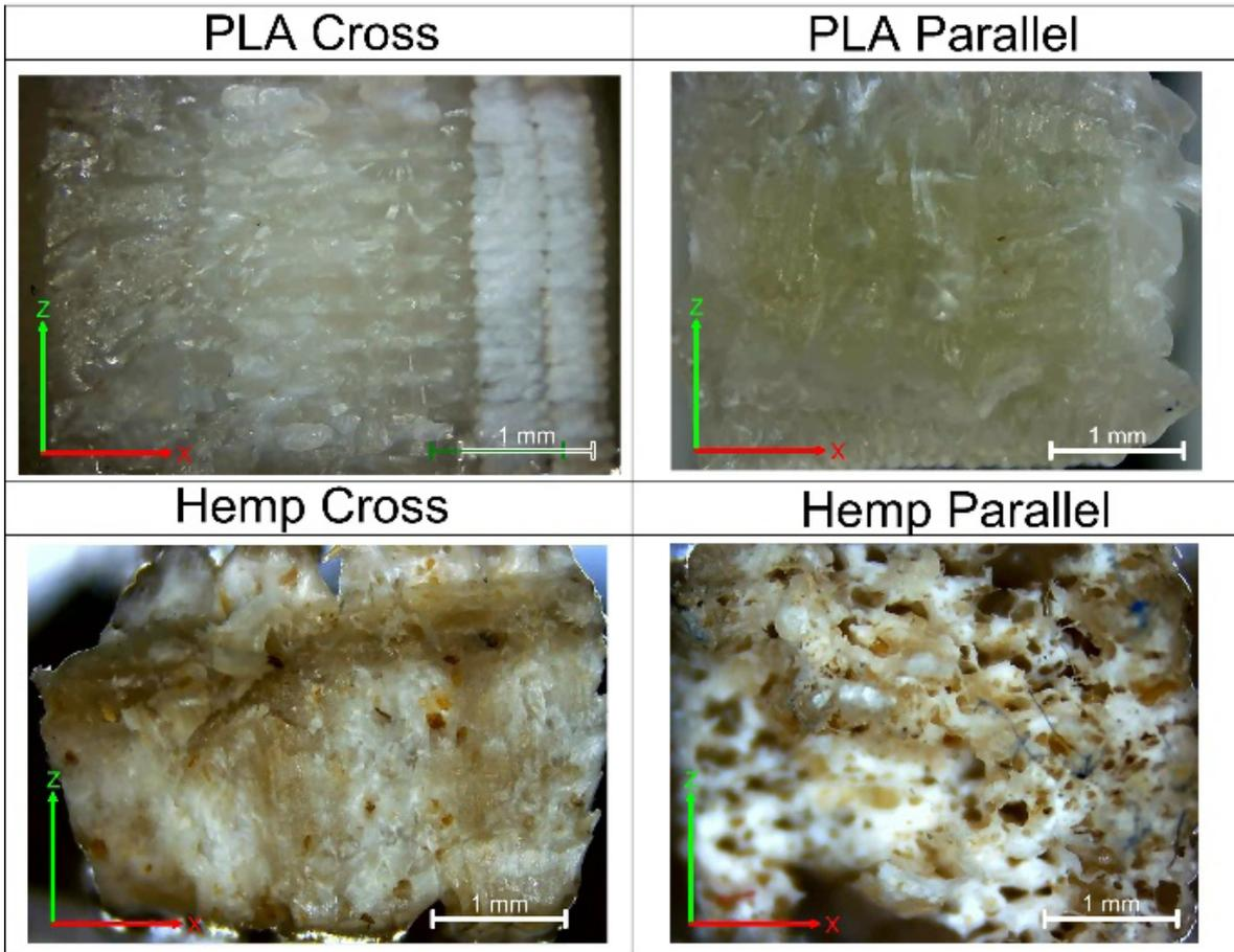
Figure 4. Optical microscope images.
