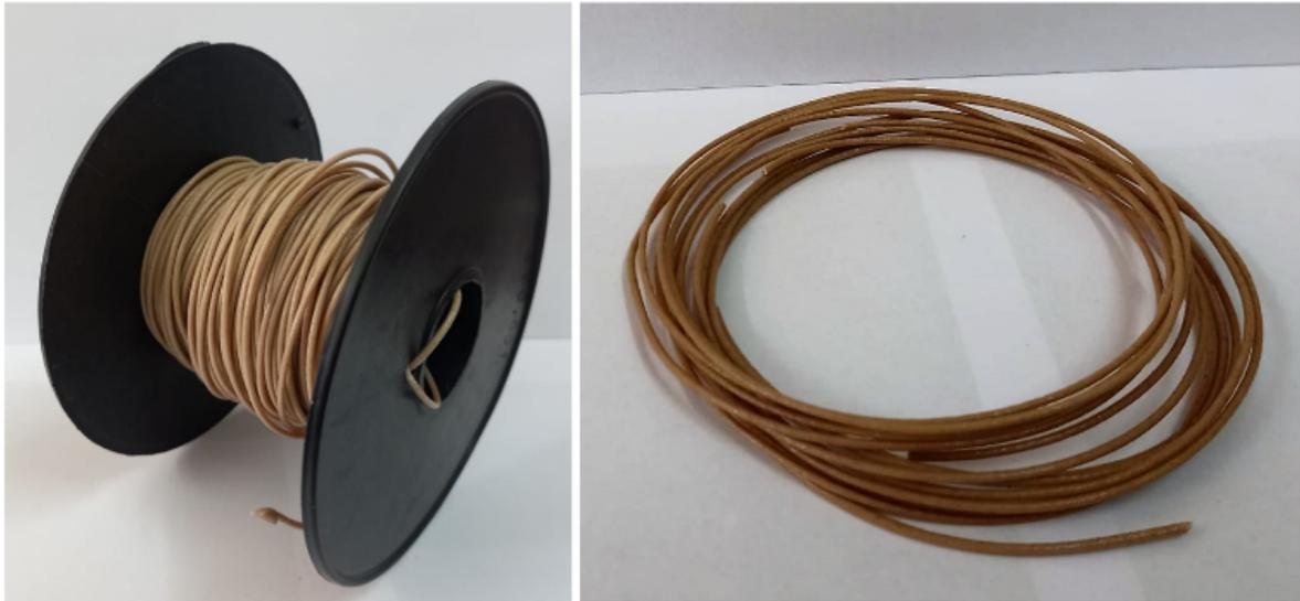
**Figure 2.** Hemp reinforced PLA filament.
