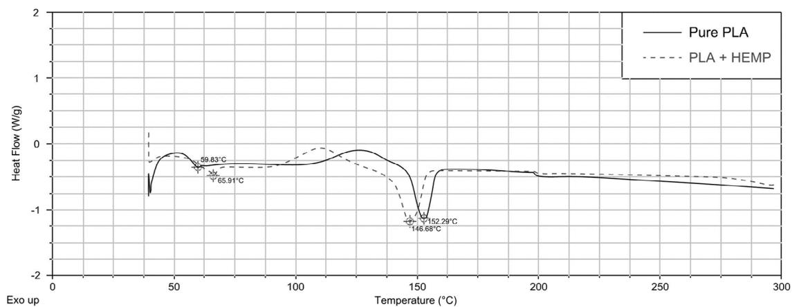
Figure 7. Differential scanning calorimetry (DSC) analysis results.
