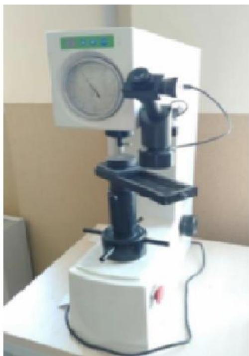
**Figure 2.** Hardness tester.
