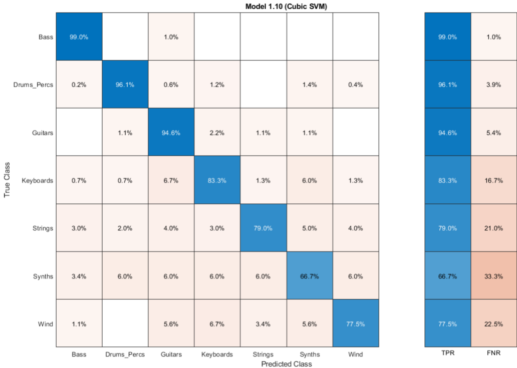
Figure-3: Confusion matrix for SVM-Cubic. In left side percentages of success and misclassification rates for each instrument family are shown in a comparative way. In the right side, True Positive Rates (TPR) and False Negative Rates (FNR) gives a general clue about misclassifications.
