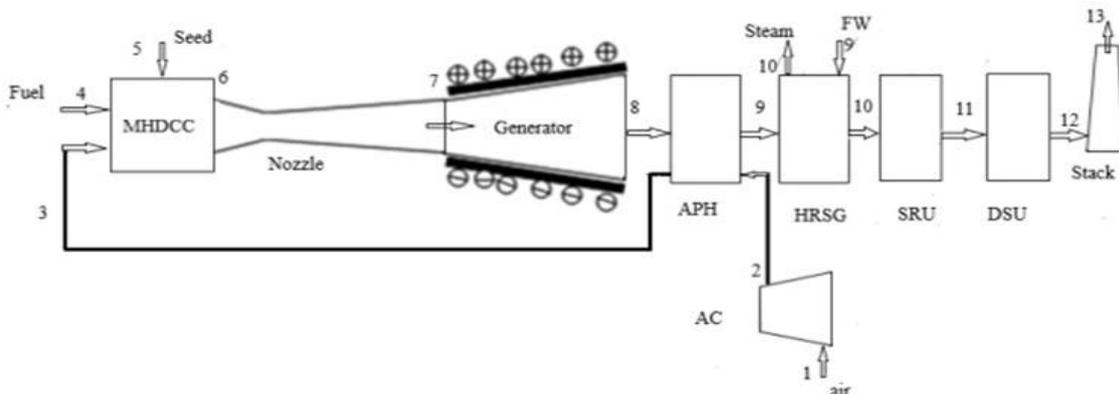
Figure 1. Schematic of the standalone MHD power plant
