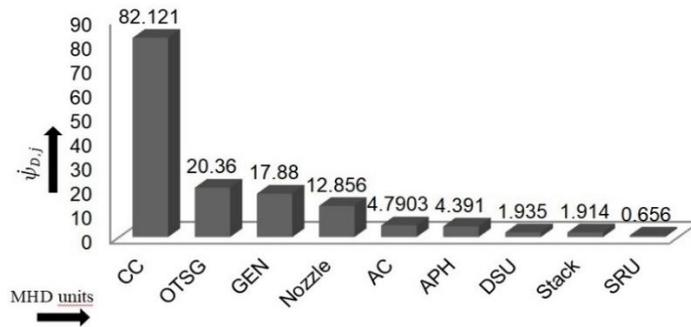
Figure 3. Allocation of exergy desolation rate (MW) in different units of the MHD system.
