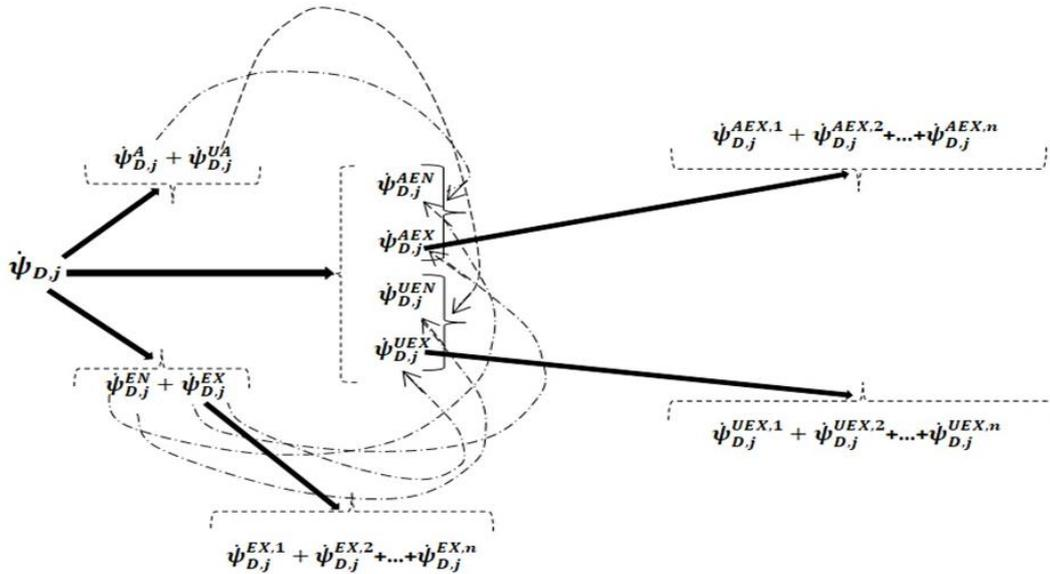
Figure 2. Division of exergy destructions inside the  $j$ th unit of the system [26].
