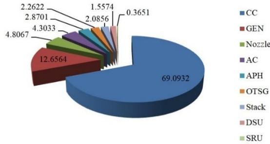
Figure 5. Percentage comparison of the endogenous exergy desolation in the *j*th unit of the MHD system.
