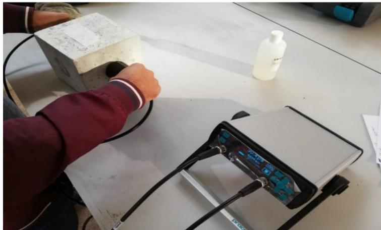
**Figure 2.** Ultrasonic transmission rate determination
