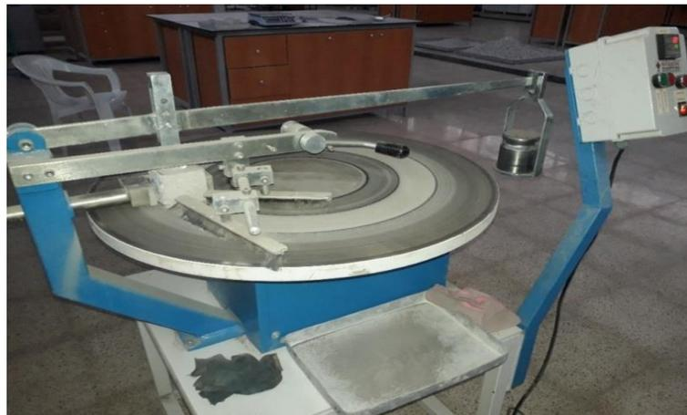
**Figure 1.** Böhme experimental setup
