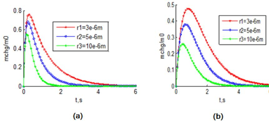
**Figure 2.** The amount of charged particles located in the studied space, respectively. (a)- at a current density  $j = 10^{-4} A/m^2$  and (b)- at a current density  $j = 5.10^{-4} A/m^2$
