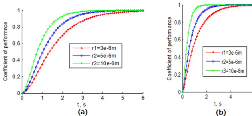
**Figure 3.** The dependence of the coefficient of performance of the active zone of corona discharge, respectively (a)- at a current density  $j = \frac{10^{-4} A}{m^2}$  and (b)- at a current density  $j = \frac{5.10^{-4} A}{m^2}$
