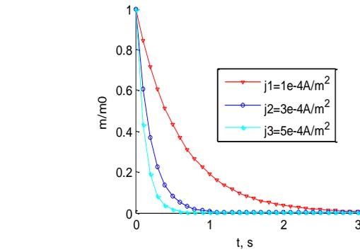
**Figure 1.** Changes in amount of charged particles as a function of the active zone corona for different values of ion current density
