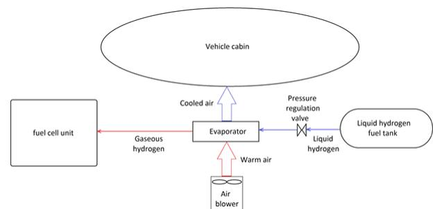
Figure 1 Layout of the AAC system for LH<sub>2</sub> powered FCVs
