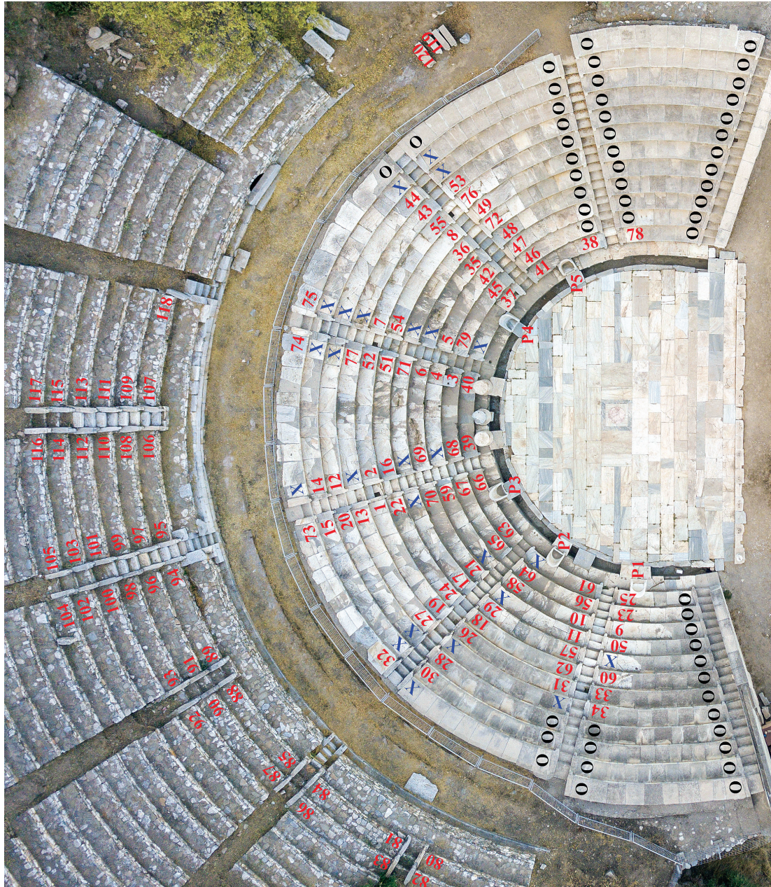
FIG. 3 Distribution of the prohedriai and lion's feet in the theater. (X; lion's feet excluded from the evaluation due to poor condition). (O; Replicas of lion's feet created within the scope of the restoration project).
