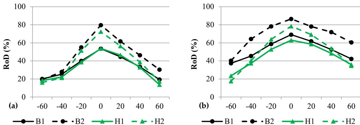
Figure 9. RoD values for arithmetic mean speed in (a) FF and (b) OSF traffic regime
