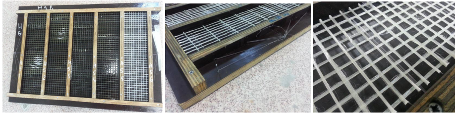
Figure 6. Special molds with holes for structure production from epoxy resin coated filament or hybrid yarn
