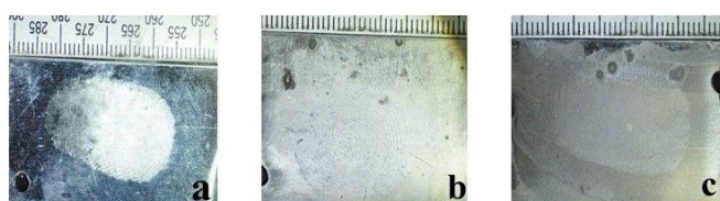
Figure 3. Fingerprint Development on Metal Surfaces; a) 12 months trace development in the air environment, b) 90 days trace development in the freshwater environment, c) 30 days trace development in the saltwater environment
