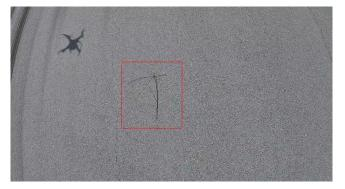
Figure 5 Foreign object (bush) detected on the runway
