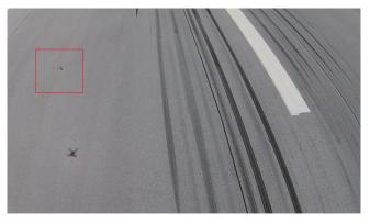
Figure 4 Foreign object (bush) detected on the runway
