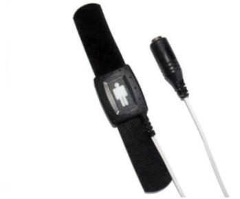
Figure 2. The body position sensor used in this study [13]
