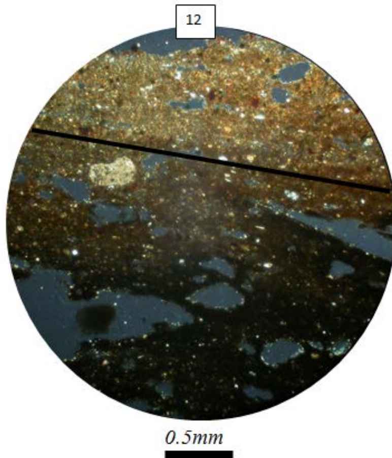
Figure (12). SEM image of Sample ES.4, 4X magnification, XPL, image captured from the pottery edge (bright color) toward the central part (dark color). There is no compositional shift between the two parts, which might be due to chromatic shift under the curing conditions of the furnace.
