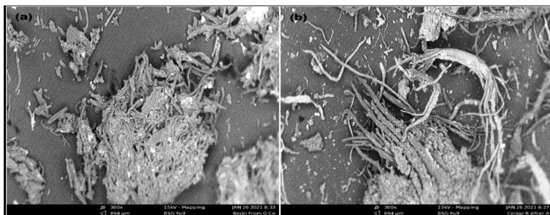
Figure 3: SEM image of (a) poly (amidoxime) ligand, (b) poly(amidoxime) ligand after \text{Cu}^{2+} adsorption.
